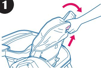
**With baby out of high chair,** squeeze recline lever and adjust seat back to 1 of 3 positions.
